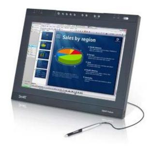
The SMART Sympodium monitor allows you to annotate on PowerPoint slides using the attached touch pen
